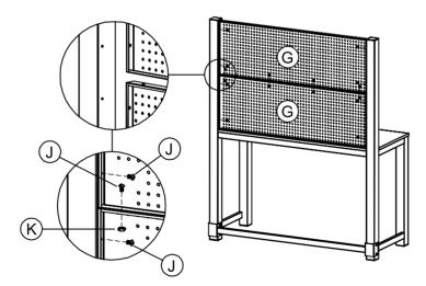
Step 4. Position the pegboards on the bench top and align with the left and right legs. Join the two pegboards using M6\*15mm phillips head bolts and M6 hex nuts. Fix the pegboards to the legs using M6\*15mm phillips head bolts.
