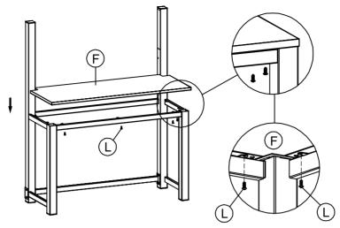
Step 3. Fix the MDF table top onto the table frame by self tapping screws as per diagram.
