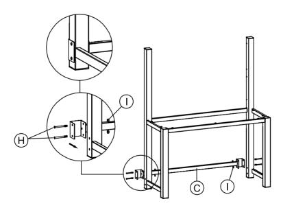
Step 2. Insert and fix horizontal back brace with M8\*95mm phillips head bolts and M8 hex nuts as per diagram.
