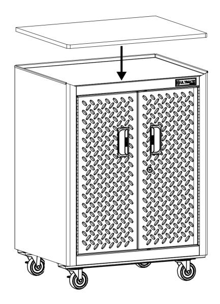
Step 2. Recover the cabinet to upright position. Place the MDF Bench top (1) on the top of the Cabinet Body.
