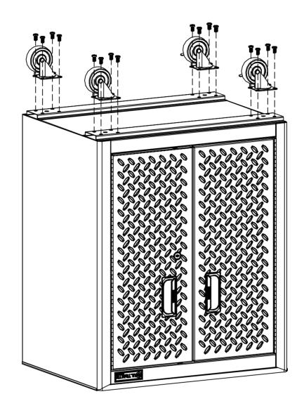
Step 1. Place the Cabinet Body (2) on the ground, upside down. Fix the castors (With Brakes) (3) on one side of the Cabinet Body and fix the Castors (4) on the other side, using the M8 x 15mm Pan Head Hex Bolts (5) provided.
