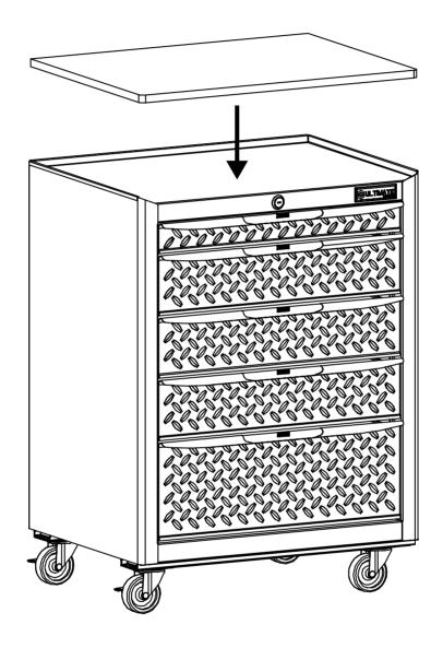
Step 2. Recover the cabinet to upright position. Place the MDF Bench Top (1) on the top of the Cabinet Body.
