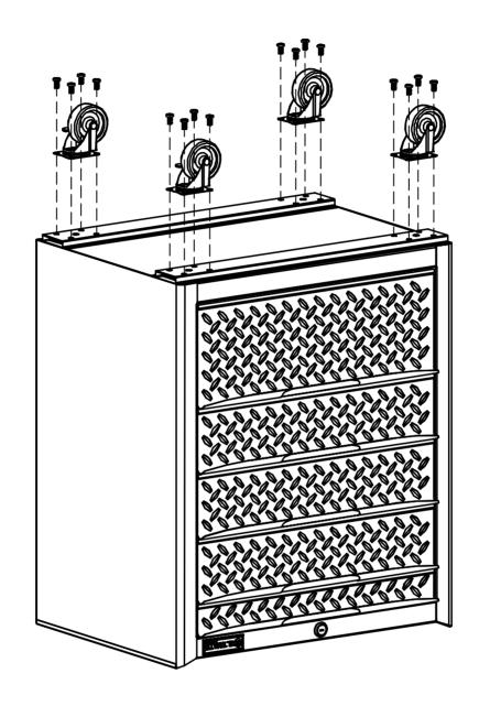
Step 1. Place the Cabinet Body (2) on the ground, upside down. Fix the castors (With Brakes) (3) on one side of the Cabinet Body and fix the Castors (4) on the other side, using the M8 x 15mm Pan Head Hex Bolts (5) provided.
