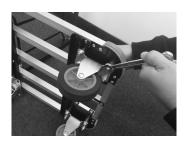
Using a spanner and socket, fix the four wheels onto the frame using the provided fixings. Locknuts are used to help prevent loosening during 'bumpy' transportation, be sure to check these from time to time and make adjustments if necessary.
