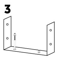
Position base frame, insert the dynabolts into the 2 holes and secure by tightening.
