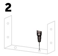
Take base frame away and pre-drill holes using a 10 mm masonry drill bit.
