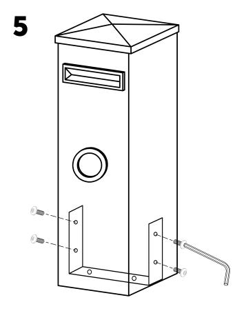
Place letterbox body over frame. Attach using the bolts provided.
